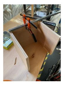
**Step 5**—Lie the "C" frame on it's side and align the X-Rail against the frame. Ensure the side of the frame that has been aligned is the side opposite the "face" of the carriage. It's not a bad idea to clamp this thing in place.
